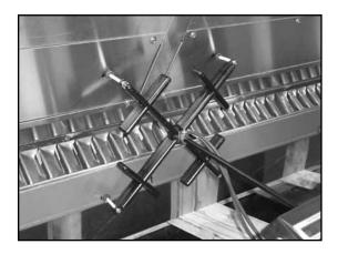
After the appropriate number of readings have been taken from the inlet slot of the hood, an average reading can be calculated by summing the velocity readings and dividing the total value by the number of readings taken.
